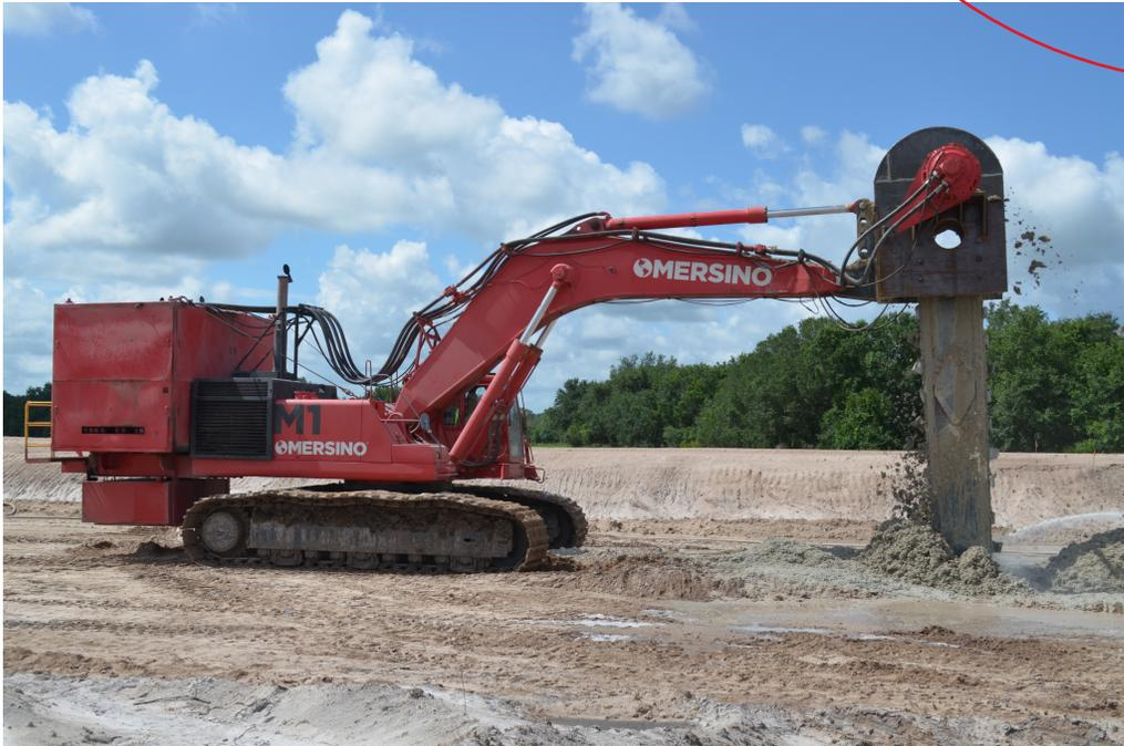
Mersino's One-Pass Trencher is highly precise equipment to perform one-pass trenching services. Laser guides and GPS systems allow for accurate installation along irregular grades for maximize efficiency. The GPS system allows for the precise installation of cable and utility lines for accurate mapping of underground locations in the future.
